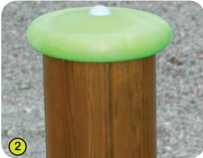
2- **The 125mm round posts** are made of laminated timber, which have not been treated with chrome or arsenic. Splinter-free, the laminate provides great strength and dimensional stability. The posts are protected from wear and tear caused by fungi, insects and termites. The caps are made of injection moulded polyamide.
