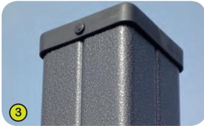
3- **The central posts**, which measure 95 x 95 mm, are made of galvanized, lacquered steel. The two-tone grey graining finish has a slightly undulating surface for increased scratch resistance. The caps are made of injection moulded polyamide.
